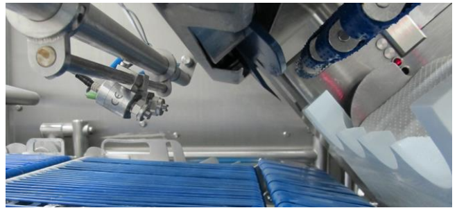
PhageGuard Listex is applied at the point of slicing which potentially is a vulnerable point of contamination.
